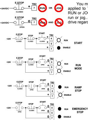
You must have +24VDC (all voltages are relative to TB1 terminal 16) applied to TB2 terminal 7 (Emergency Stop input) before attempting to RUN or JOG. You must maintain +24V on TB2 - 7 as long as you want to run or jog.. Removing +24V from the Emergency Stop input will stop the drive regardless of whatever other inputs may be energized.
