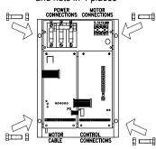
Mount a Model 1000 series drive of the NEMA 1 style with the fuses at the top. Do not block air flow around the unit. Free air must flow up through the fins on the back of the drive.
