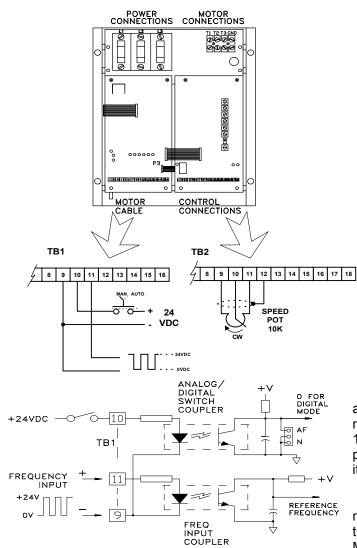
Apply +24VDC to TB1 terminal 10 (TB1-10) with respect to TB1-9 to operate the Model 1000 with a digital reference. Terminal 9 on TB1 is NOT the same as drive common, so a jumper from TB2-8 or TB2-17 will NOT switch to digital mode unless you connect TB1-9 to a drive common terminal (TB1-16).
