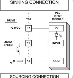
Most of the signals are +24 VDC or 48 VDC (positive and negative 24 VDC supplies for control), or +10 VDC for speed. You may also use computer generated frequency signals for speed in the DIGITAL mode.
