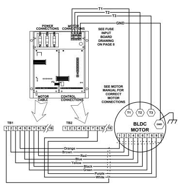
Connect the motor lead marked T1 to the T1 terminal on the drive. Connect the T2 lead to T2 on the drive, and connect T3 to T3. Other connections to T1, T2, and T3 at the motor will vary with the motor. The motor will not operate correctly if the power wires from motor to drive are not in the proper order.
