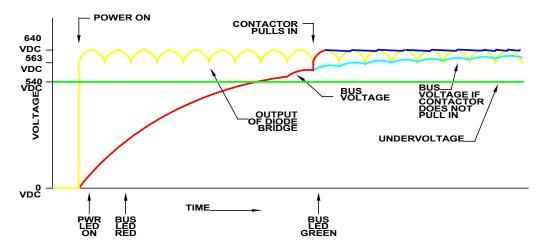
The bus voltage can be observed with a voltmeter connected to the POSITIVE BUS and NEGATIVE BUS terminals on the Capacitor Board. This board is located on the right sidewall of the drive behind the front panels (see page 28). The Bus terminals are near the top of the drive. BE CAREFUL. THESE TERMINALS MAY HAVE POTENTIALS UP TO 800VDC!!
