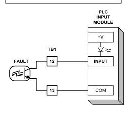
A "sourcing" connection turns on the PLC module by supplying power to it. The second figure shows a sourcing connection. Notice, however, the inverted sense, that is, when the transistor turns on, the input is not.
