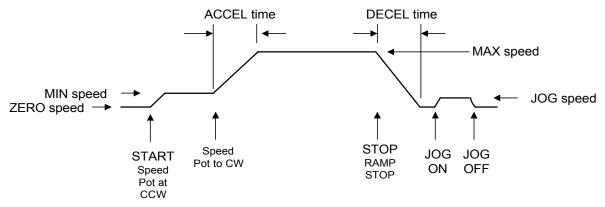
With a standard speed pot connection (see page 21), the MIN pot on the Speed Controller board is actually a minimum reference level. When the drive is started in the RUN mode with the speed pot fully counter-clockwise (CCW, or 0%), the speed reference will be whatever is dialed in on the MIN speed pot.
